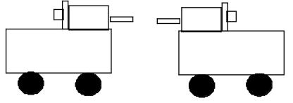
The force probes should be securely fastened to the carts.
